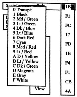
Enter the color codes you would like. The first being the foreground color and the second being the background. After pressing <ENTER> the screen will revert back to the screen prior to this one, where you can VIEW this combination. This configuration is for the screen and text colors.
