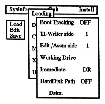
You select pressing the first letter of the desired function. In pressing "B", the BOOT TRACKING (knowing where the programs were loaded from) is switched from on to off and back on again. Leave it ON, if all the Funnelweb files are together on one disk, so you don't have to tell it where to load other programs segments from.
