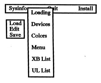
LOADING is where the primary system files are found, whether or not you have boot tracking on and which of three program segments is to be loaded immediately upon booting.
