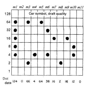
ASCII Code 92 Descender 1 m0 = Descender x 128Start column 0 + (Start x 16) End column + End
