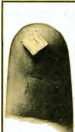
The Texas Instruments microcomputer seen in the preceding illustration is shown here in its actual size as it rests on a person's fingertip. Thousands of infinitesimal transistors are crammed onto this simple computer-on-a-chip. (Courtesy of Texas Instruments, Inc.)
