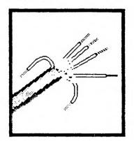
Trim back the outer insulation <sup>3</sup>/4 to <sup>7</sup>/8 of an inch. Then trim back the insulation on each wire <sup>3</sup>/16 of an inch.
