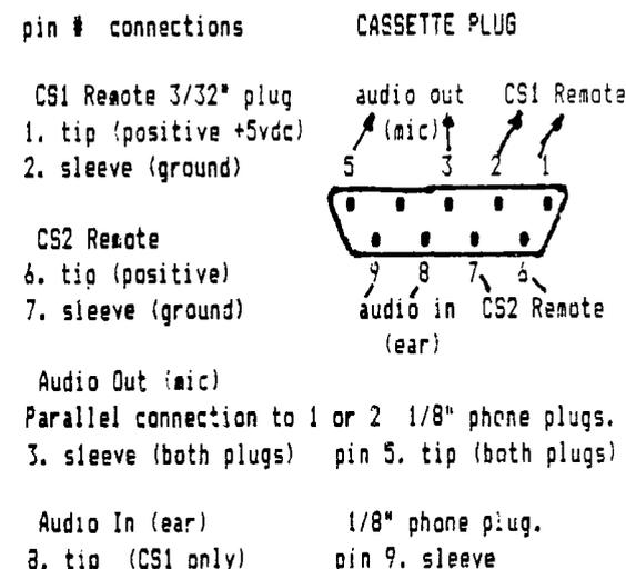
The remotes are ordinarily on, presenting a closed circuit to the cassette. This corresponds to CALL LINK("CS1",1) or SBO 0 in the program. The system turns off the cassette only when a file is OPENed. Until the FROM tape routines are entered-- CLD, SAVE, OPEN -- you may rewind the cassette. If the console is turned off, the circuits are open. The remote circuits protect the CPU with the infrared optocoupler TIL 119, 'photodarlington'. The circuit can handle 5vdc with complete safety.
