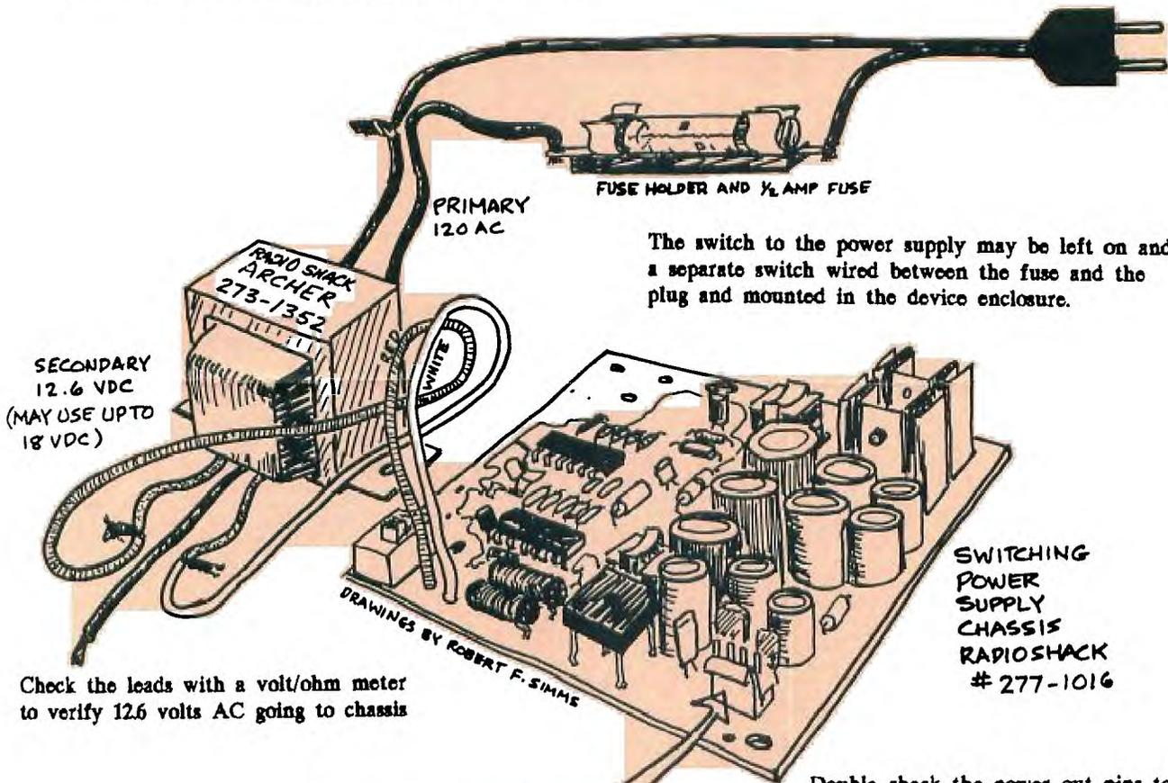
Check the leads with a volt/ohm meter to verify 12.6 volts AC going to chassis
