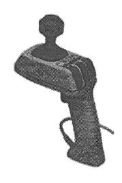
One joystick comes as standard equipment with each MBX system. A second joystick is listed in T.I.'s last 99/4A price list for \$29.95 and can be plugged into the second joystick port on the control box. This would give each of two players their own separate joystick. In actual use of the MBX software modules a second joystick isn't really needed. Only one player at a time uses the joystick. The
