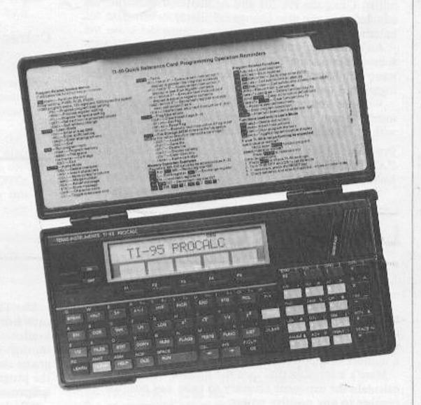
This program was first run without assembling (key sequence: RUN, PGM), and the execution time was approximately 15 seconds. The program was then assembled and run (key sequence: 2nd, ASM, RUN, PGM) with execution time reduced by more than half (6.5 seconds). In the unassembled program, the calculator had to scan through all NOP's before transferring control to the correct labels. In the assembled program, control is transferred directly to the absolute address.
