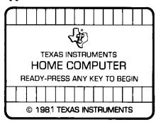
Then, press any key. The master selection list comes on the screen, showing TI BASIC as the first choice. Press the 1 key to select TI BASIC. The screen then indicates that the computer is "ready" to respond to BASIC commands and programs.
