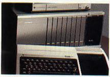
The RS232 Interface Card, with up to two serial ports, lets you hook up to a wide range of serially formatted accessories. It also has one parallel port to utilize a printer. The Memory Expansion Unit increases the Home Computer's random access memory from 16K bytes to 48K bytes.
