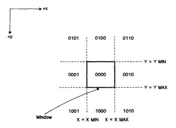
Figure 7-11. Outcodes for Line Endpoints
