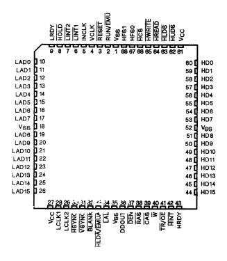
Figure 2-1. TMS34010 Pinout (Top View)
