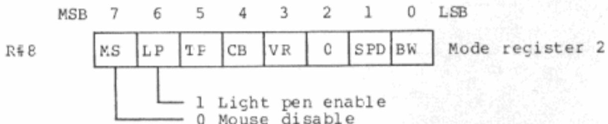
In addition, if you want to enable an interrupt when the light pen has detected light, set bit 5 of register R#0 to 1. This interrupt is reset if status register S#1 is read.
