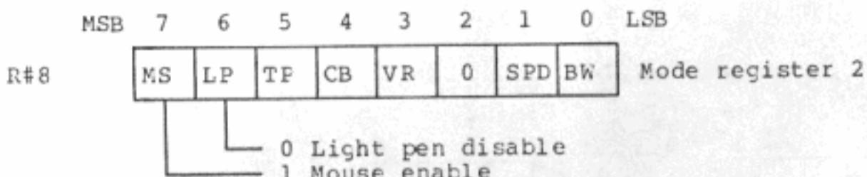
When bit 7 of register R#8 is set to 1, the direction of the Color Bus is automatically changed to input.
