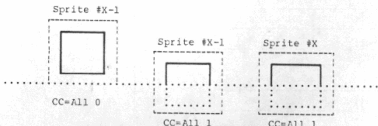
For the portions of the sprite in which CC is set to 1, even if a sprite having the number which is closest to that sprite has CC=0 overlaps the sprite, the collision is not detected. For overlapping sprites, a logical OR is done on the color codes for display.
