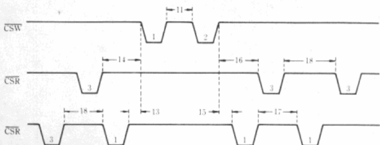
Note: The numbers n (where n = 1, 2, 3) marked in the pulses show the byte order (1st, 2nd, 3rd) sent from the CPU.
