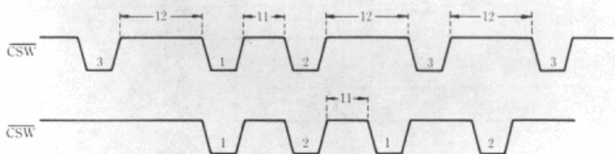
Note: The numbers n (where n = 1, 2, 3) marked in the pulses show the byte order (1st, 2nd, 3rd) sent from the CPU.
