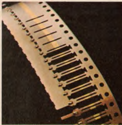
Clad metal strips are stamped into contacts by high speed presses.
