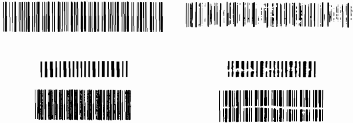
Figure 6. Good- and Poor-Quality Bar Codes
