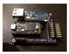
The TI-99 USB Keys adapter is built on open source hardware which makes it very easy to obtain. The end result is being able to hook up a USB keyboard to the TI and having every key mapped correctly. Now a user does not have to replace the TI keyboard to use the USB keyboard, they will both work at the same time.
