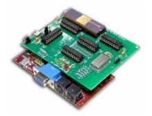
Erik Pehl has developed a device that allows a user to have a CLONE of the TI-99/4A using the TMS99105 processor and a Pepino FPGA board with XC6SLX9 chip.
