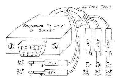
The plug is a standard '9.WAY.D. SOCKET.'. The contacts ,numbered one to nine, are 'HOLES' into which the pins of the plug can be inserted. It costs about £3.
