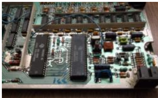
tms 9929a chip before removal
