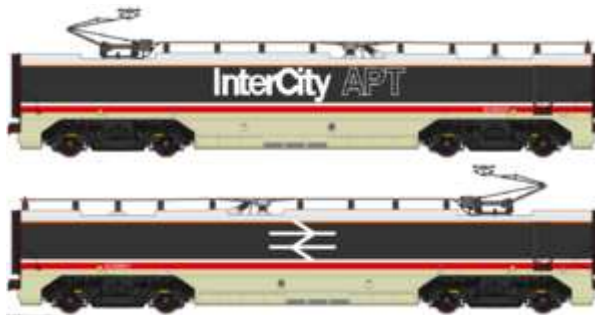
APT-P Non-Driving Motor (NDM) unit, with Stone Faiveley AMBR pantograph
