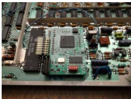
F18a board in place without cable.
