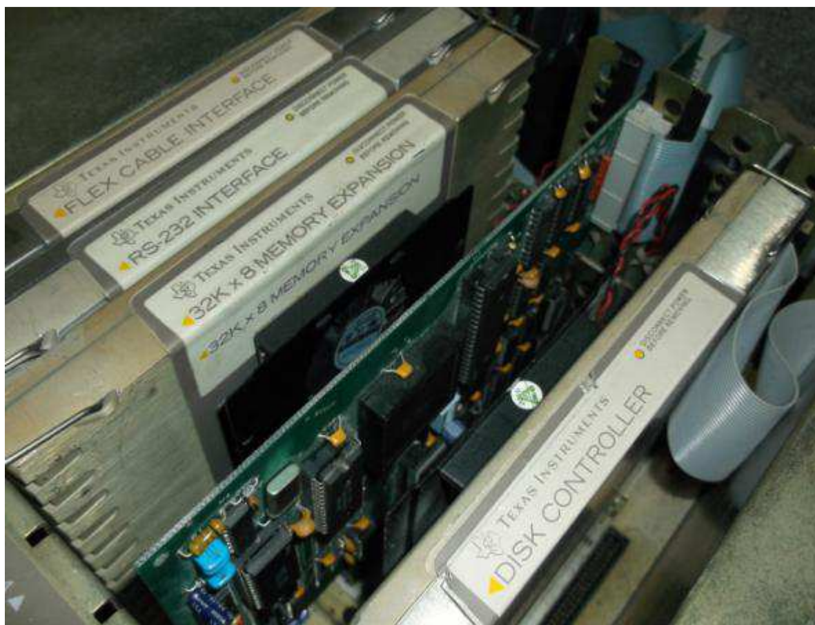
My PEB. With 1990s. HFDC version H11 card with low power cool air fans either side.
