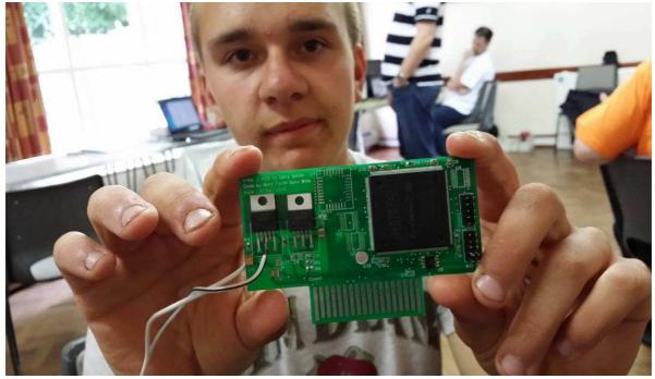
This is a new cartridge for the Texas. It's really a processor in the big square chip and has four cores which means there are really four processors in one. It doesn't work in machine code like a normal processor, it runs the Forth language. It does over 200 million instructions a second.
