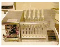
Ready for the main cover to be installed. I chose to install the power supply cover (or wind tunnel) on the chassis first, to ease main cover installation and also to see that everything fits well. Remainder of card cage and the plastic floppy drive support installed as well.
