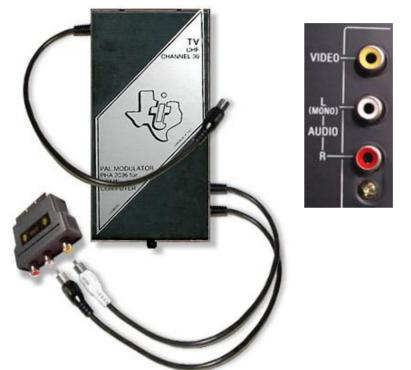
Double check all the connections and take care that the new cables installed do not touch others components. Insulate them if necessary. Cut a small part of the metal case to route the cables outside the modulator and close it.
