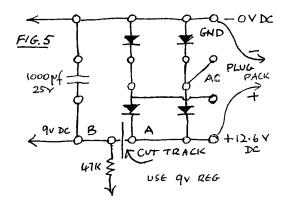
I have built the RGB Interface and powered it by both the 16VAC plug pack and the full wave centre tap circuit and both gave a bright clean screen. However, I have not been able to check the 9V version in regard to its performance on the screen, but the regulator circuit does output a steady 9V as predicted.  $\boldsymbol{o}$
