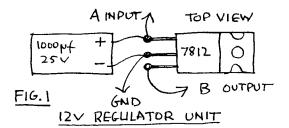
See Figure 1 as to how to combine these two items into a single unit with 3 leads attached. (INPUT,GND,OUTPUT). There is one change to the PCB. One track to cut. Figure 2 indicates where to make this cut.
