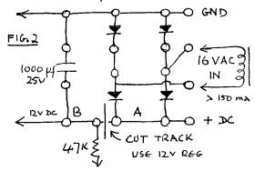
Mounting the regulator is not difficult. The metal tab of the 7812 is as one with the centre common pin and can be bolted directly to the metal housing or other convenient location, and is at GND potential. The three leads can then be soldered to the points indicated in Figure 2.
