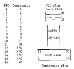
Note: N/C connections are cut off at Centronics plug.
