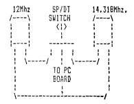
The diagram better explains the circuit. The switch can be mounted in the cooling vent on the top of the console. It seems that you can switch back and forth between crystals while a Basic program is running.
