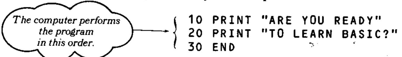
Also, you may be wondering why we numbered the lines in increments of ten (10,20,30,etc.). Well, we could just as easily have numbered them 1,2,3. By using increments of ten, however, or other spreads like 100,200,300, etc., we can go back and insert new lines if we want to expand the existing program, and we don't have to retype the whole program! (We'll cover this clever trick when we discuss editing a program.)
