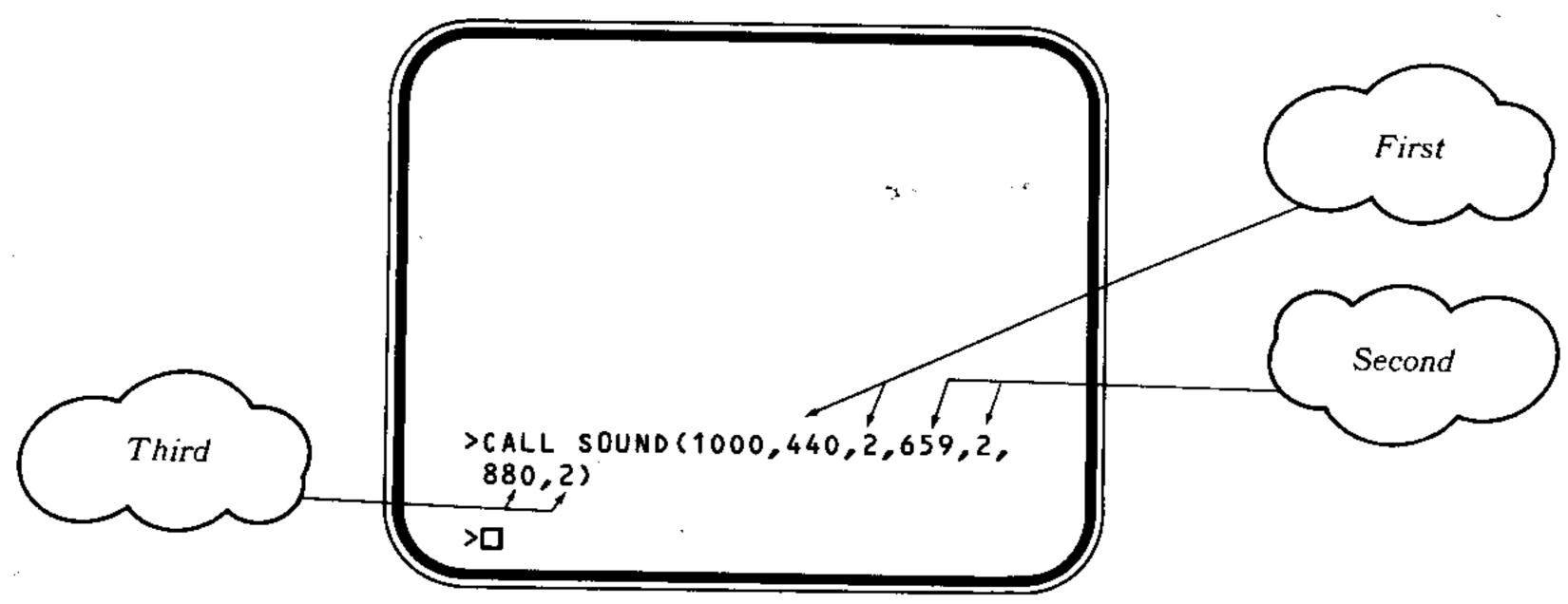
(Part of this CALL SOUND statement extends to the second line, since TI BASIC uses only 28 printing positions per line. This gives large, clear, readable text on the screen.)
