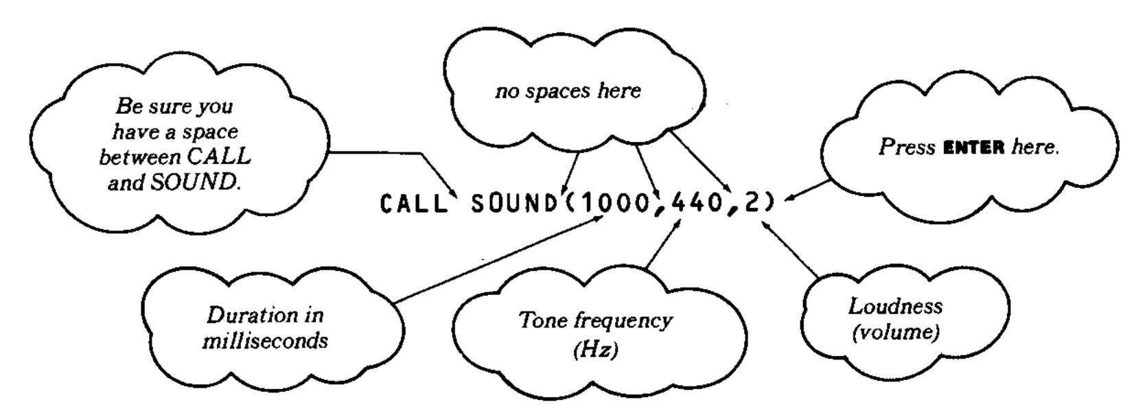
Notice that the three values that control the sound are enclosed in parentheses following the words CALL SOUND. This example will produce a note of 440 Hz (A above middle C) with a duration of 1000 milliseconds (one second) and a volume of 2 (quite loud!).
