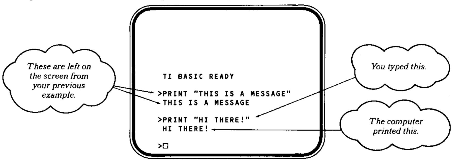
Did you notice the way the lines moved up on the screen when you pressed **ENTER** and again when the computer finished printing its line? This procedure is called *scrolling*. The cursor tells you it's your turn now and shows you where the next line will begin.
