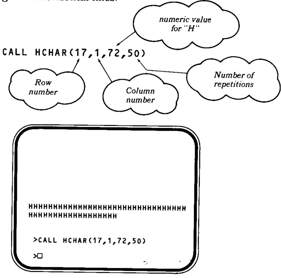
Again the printing filled one line (horizontal, this time) and then started over on the next line. Count the H's. If you see only 28 in the full line, columns 1 and 2, 31 and 32 do not show on your screen, and you should use only columns 3 through 30 to avoid losing part of your graphic design.
