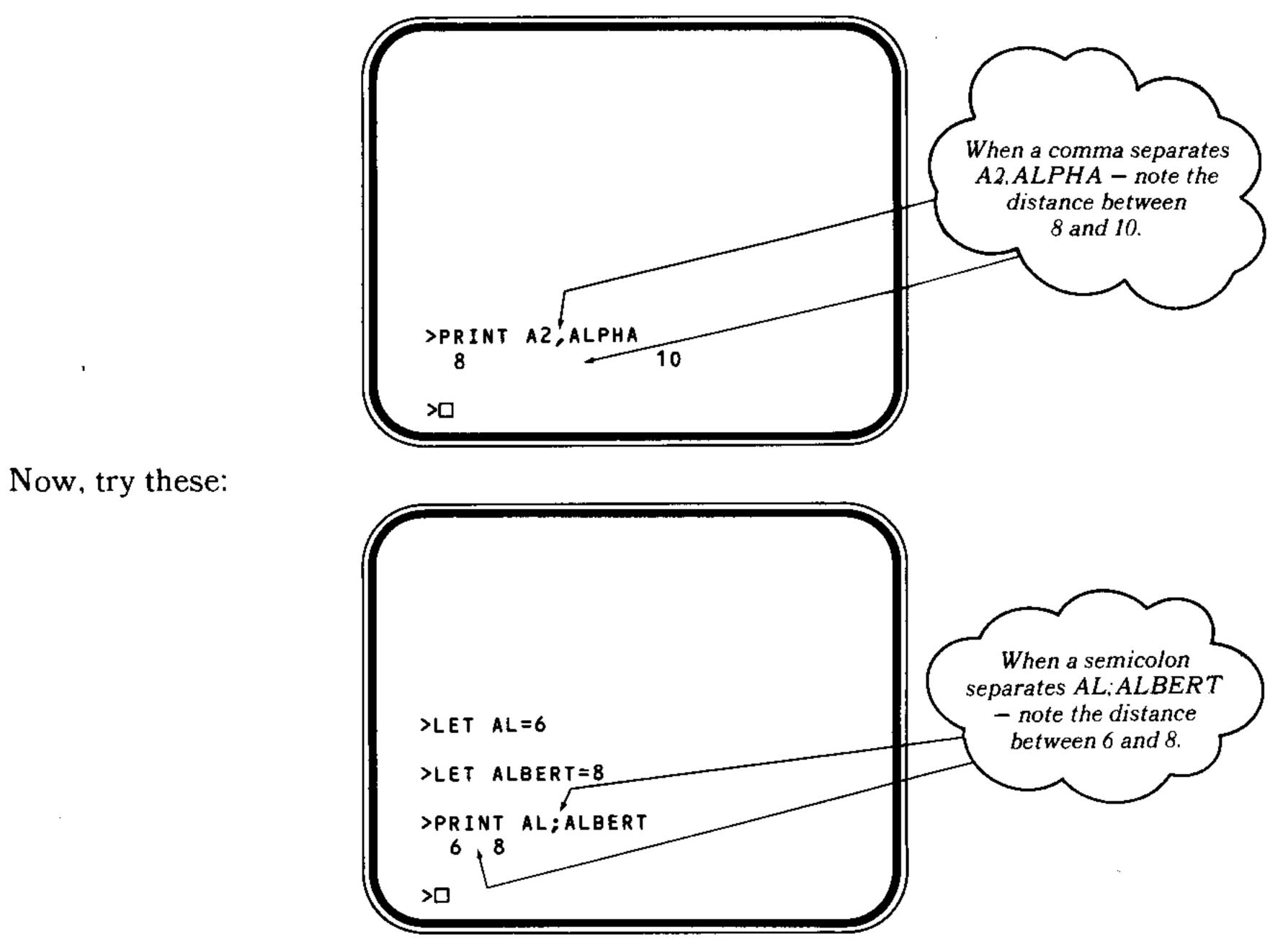
The computer divides the display screen into two horizontal zones. When you use a comma (,) between two (or more) variables in a print statement, you are telling the computer to print the values in different zones. On the other hand, the semicolon (;) instructs the computer to print the numbers close together.
