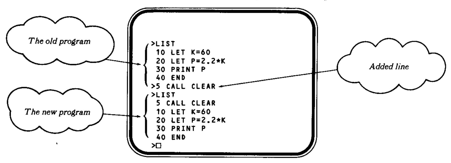
Compare the two programs on the screen, and notice that the computer has automatically placed the new line in its proper order. Run the program again to see the effect of the added line.
