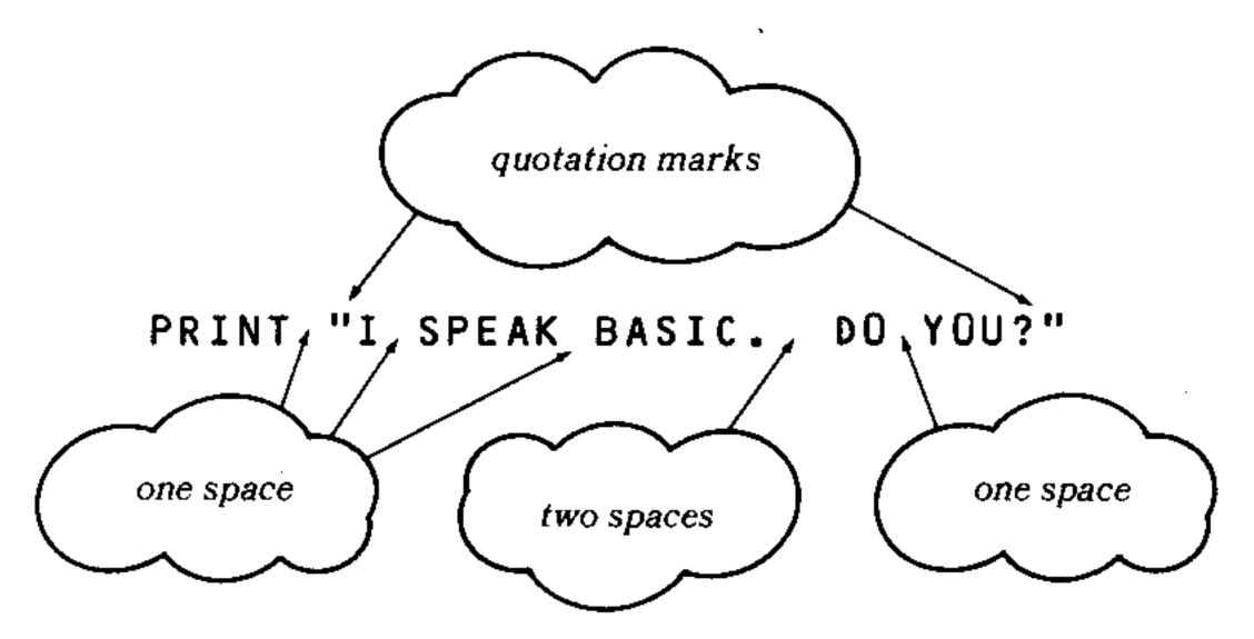
(When you run out of room on a line, just keep typing — the computer will automatically "scroll" to the next line.)
