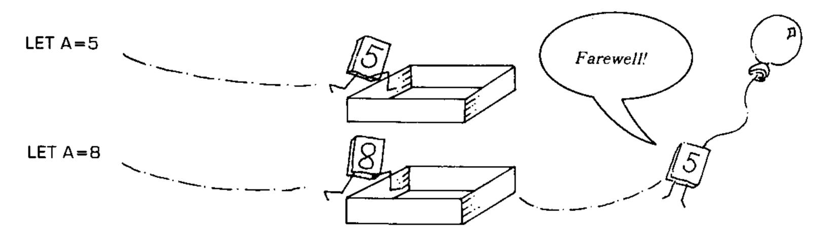
The value of A is no longer 5. The 5 has been replaced by the value 8.
