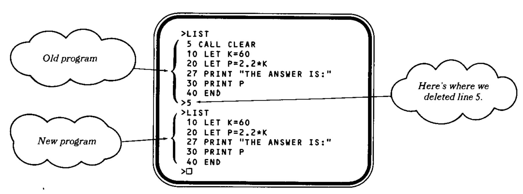
That's all there is to it. To remove a line, type the line number and press ENTER. The computer will then delete the line from program memory.
