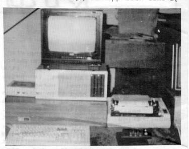
Gary Bowser. The system has a set of new circuits, a full sized keyboard and an altered operating system programmed into the lower 8k memory bank. We expect some interesting work to come out of this. We'll keep you posted as Garys work has bearing on another project in progress elsewhere.
