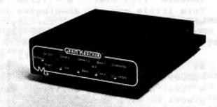
One program allows you to move the TI Writer Editor and Formatter into the GRAMKRACKER for instant loading... no more waiting for the disk access to load. Same with the Editor and Assembler programs. Another utility alters EXPLORER to work with different types of GRAM (Graphics Random Access Memory). You can also have TI Writer or the Editor Assembler loaded into the unit along with Extended Basic or another module of your choice.
