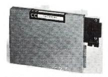
RS232 INTERFACE CARD: The CorComp design reduced the chip count of the TI card by approximately 20% increasing reliability with a reduction in
