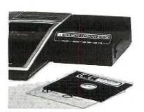
RS232 STAND ALONE: The little black box plugs directly into the side of the 99/4A. It may be purchased with one or two serial ports and one parallel for interfacing with printers and modems.
