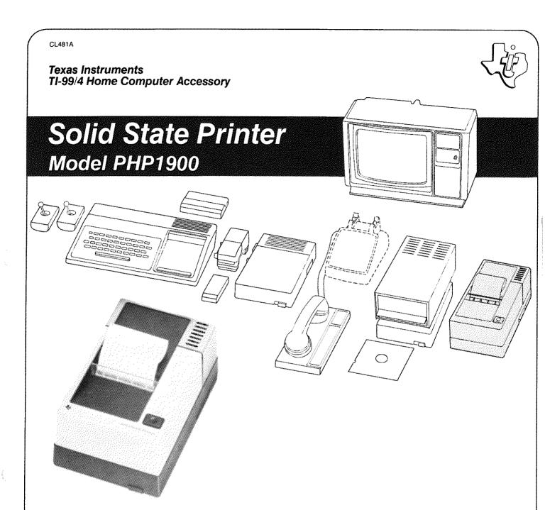
The Texas Instruments Solid State Printer permits printing of data in a 32-column, 5 x 7 dot-matrix character format at a speed of 30 characters per second. It is controlled from TI BASIC for printing results and can list programs from the computer memory. Spacing between lines can be varied under program control, and special characters using the 5 x 7 matrix format may be defined in user programs.
