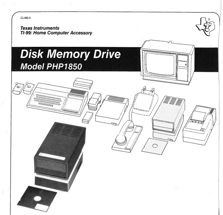
The Texas Instruments Disk Memory Drive is a minifloppy disk mass storage system with a 1 to 3-disk memory drive capability. Use of the TI Disk Memory Drive requires the TI-99/4 Disk Drive Controller (Model PHP 1800).
