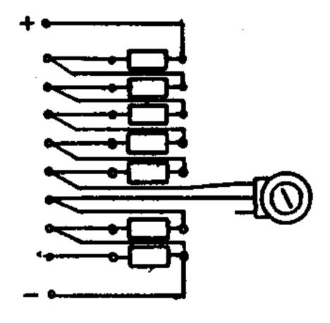
This resistor ladder can be built on a project board and connected with a cable to the socket. We used 1K ohm for the 7 resistors and a 1K variable. You can use anything you might have on hand, but be careful not to short out the + directly to the -. There you have it. The whole system works. Now the fun begins, develop your own applications and enjoy!
