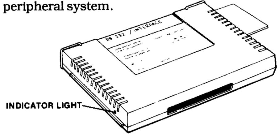
5. Carefully align the card with the desired slot and press the card firmly down into the slot.
