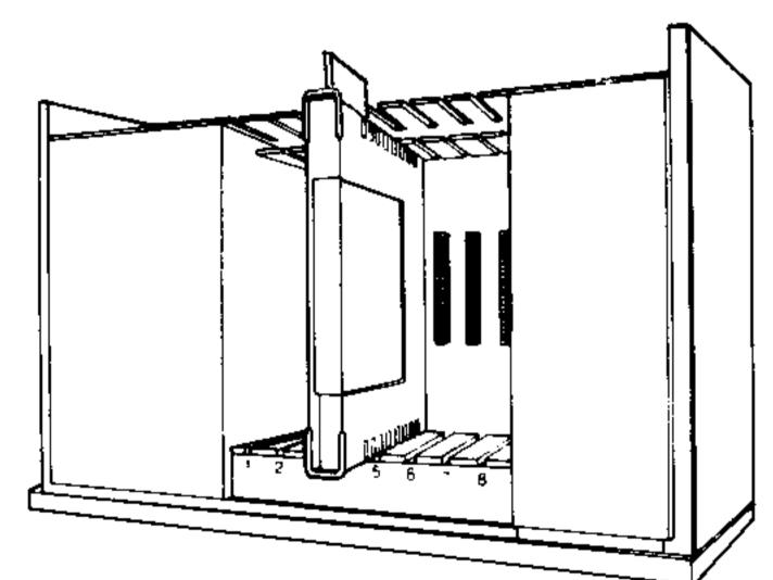
6. Replace the top on the Peripheral Expansion System by sliding the front edge under the extension on the front of the unit and firmly pressing down on the back edge of the top. Do not run the system without the top in place because the top ensures proper ventilation. *Note*: If the top does not fit properly, remove the card and realign it in the slot, remembering to press down firmly until the connection is made.
