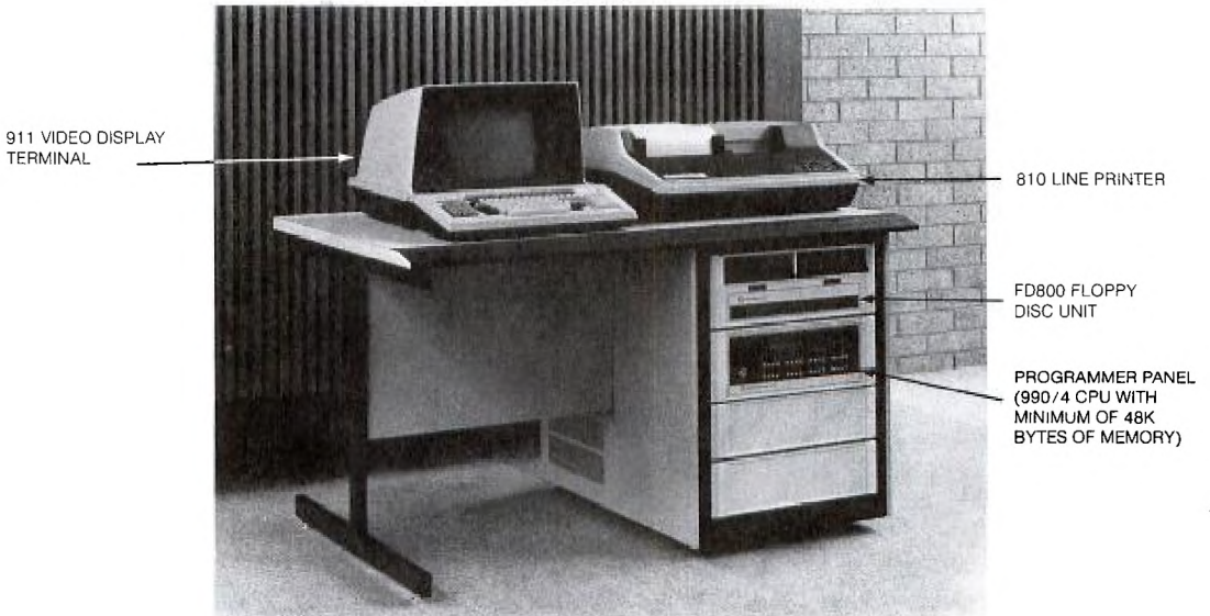
Figure 2-30. FS990 Software Development System (with optional printer)
