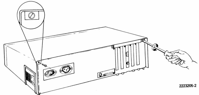
7. Remove the system unit cover by pulling it back approximately 13 mm (0.5 in), and then lifting it away from the system unit. Set the cover aside, out of the way.
