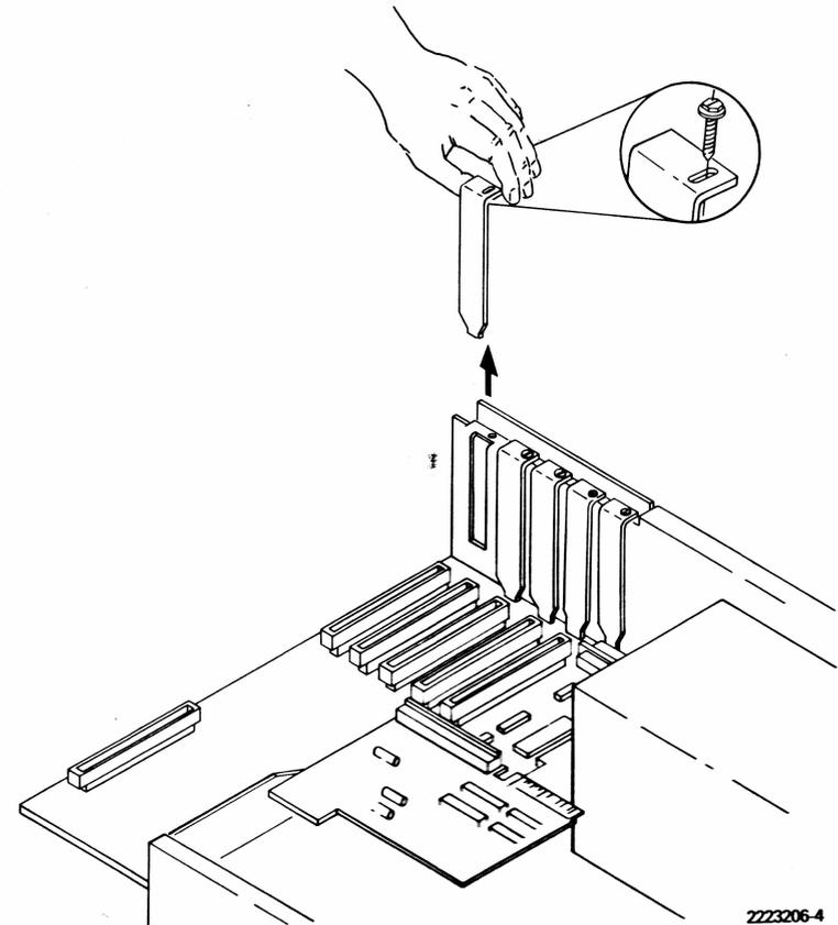
3. Gently insert the sync-async comm board into card-edge connector J5 on the system unit board. Use the slot on the rear of the system unit chassis to align the board during insertion. The locations of the connector and slot are shown below.
