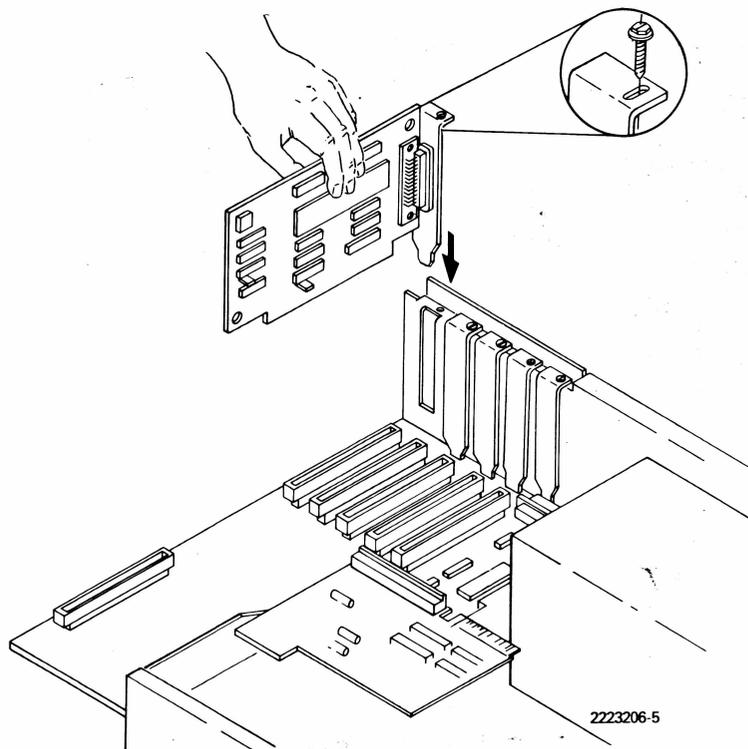
4. Align the hole on the back plate of the option board with the corresponding hole on the back panel of the system unit. Install the screw removed in step 2 and tighten, using a flat-bladed screwdriver or a 1/4-in nutdriver.
