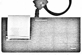
■ The PC-324 dot matrix thermal printer prints up to 24 characters per line at a speed of 48 lines per minute. The PC-324 will print the contents of each calculator's display under keyboard or program control and can provide a printed record of calculations at any time. Paper can be advanced at any time. Four AA batteries and two rolls of thermal paper are packaged with the unit. Suggested retail price: \$115.00.
