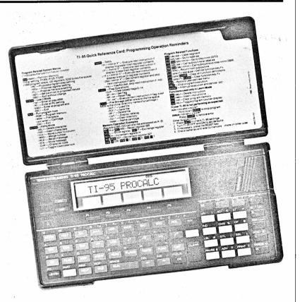
This program was first run without assembling (key sequence: RUN, PGM), and the execution time was approximately 15 seconds. The program was then assembled and run (key sequence: 2nd, ASM, RUN, PGM) with execution time reduced by more than half (6.5 seconds). In the unassembled program, the calculator had to scan through all NOP's before transferring control to the correct labels. In the assembled program, control is transferred directly to the absolute address.
