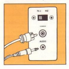
Note: Do not attach the console directly to a television set using this cable. Connection of the console to a television receiver must be made using the TI-900 Video Modulator.
