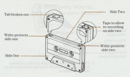
**Note:** If you need to record on a tape that has a tab missing, place a piece of cellophane tape over the tab opening.
