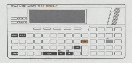
As you enter a program, the calculator does not execute your keystrokes. Instead, it stores the keystrokes in a series of numbered memory locations called *program steps*. The number of program steps is controlled by the memory partitioning of the calculator.
