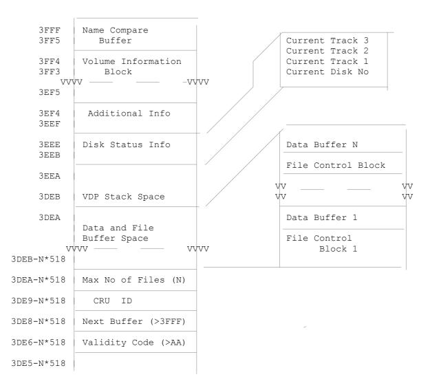
The VDP Stack area is used to simulate a stack based machine with the TMS 9900, giving the programmer the advantage of being able to use the multilevel stack oriented CALL/RETURN system, rather than the single level BL system used by the 9900 series processors. The stack can of course also be used to PUSH and POP registers and data to and From it
