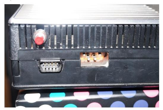
You now have a reset switch. You can mount the switch anywhere and it can be any type of momentary push-button switch as long as it is 'Normally Open'.
