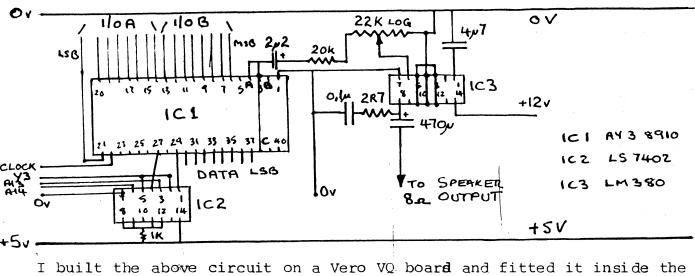
lid of my Cortex 1. Y3 is the input from IC35 on the main board and maps the PSG to F160
