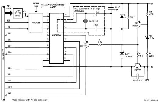
FIGURE 3. Typical System Connection Diagram
