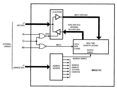
FIGURE 5. MM58274C Microprocessor Interface Diagram
