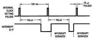
FIGURE A-1. Time Delay from Clock Setting Pulses to Interrupt is Constant
